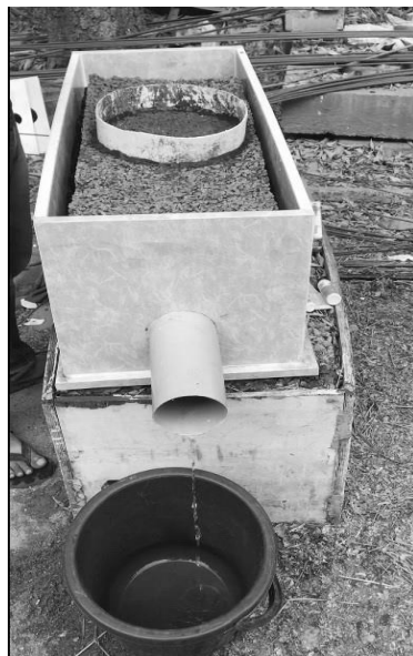
Figure 1(a). PVC miniature model 1(b). Cross section of the pervious concrete miniature model
