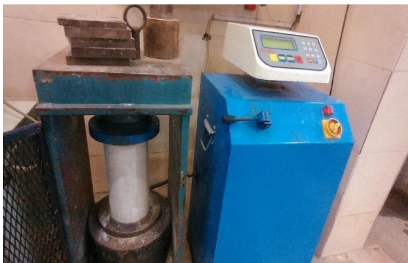
Figure 4. Uniaxial compressive strength test on standard cylindrical test piece
