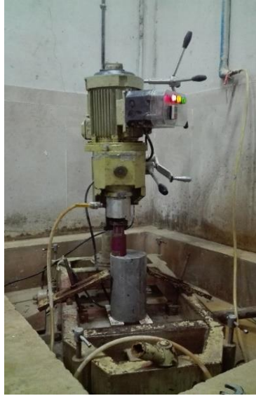
Figure 1. Coring of a standard cylindrical test.
