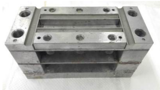
Figure 5 Mould for fibre pull-out test specimen
