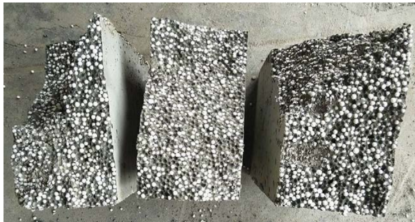
Figure 7 Even distribution of EPS among grout in blocks of Mix 4
