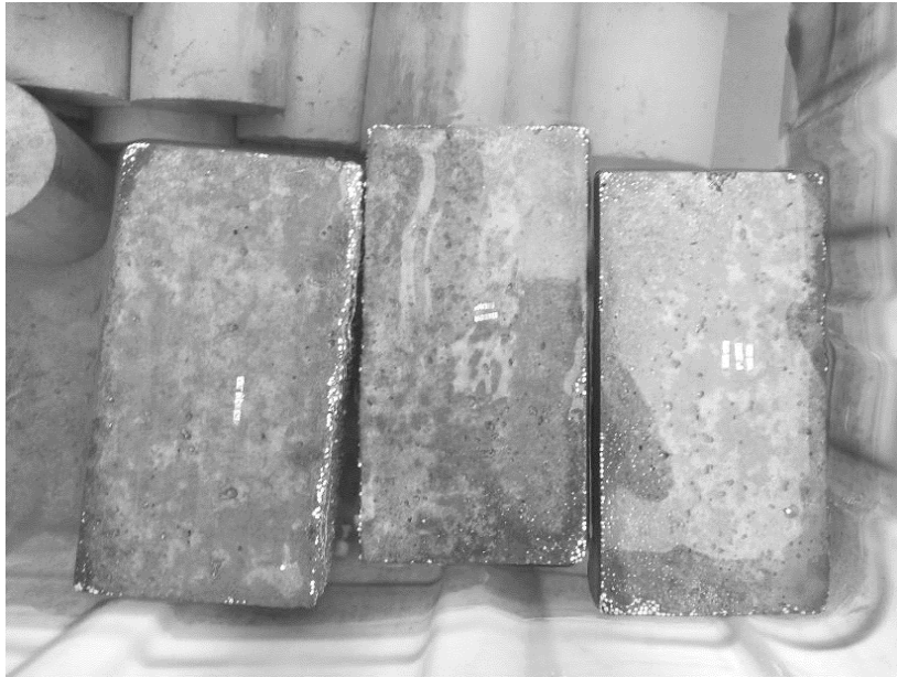
Figure 6 Blocks of Mix 4 floating on water
