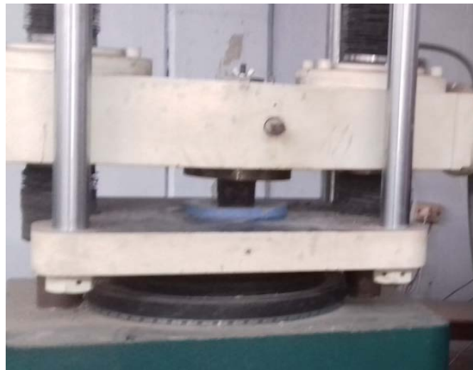
Figure 1 Compressive strength testing
