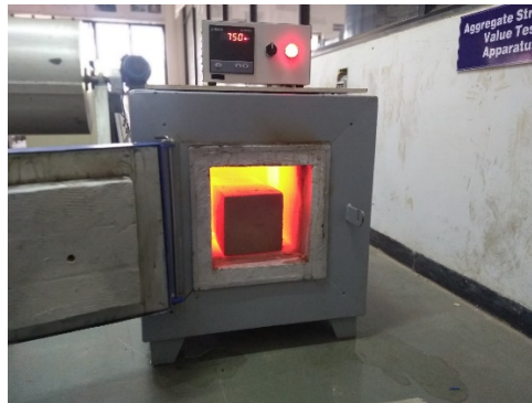
Figure 1 Furnace used for testing cubes at elevated temperatures
