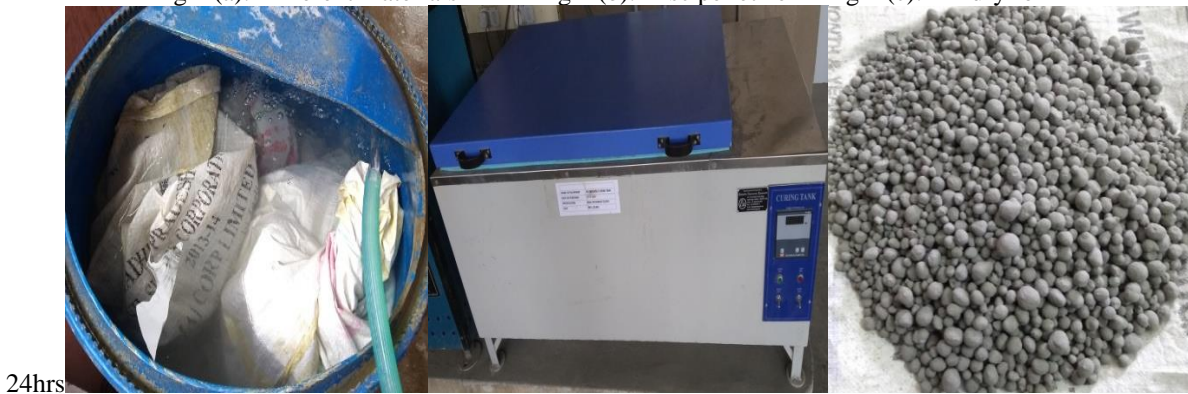
Fig 1 (d). Cold-bonding Fig 1 (e). Accelerated curing tank Fig 1 (f). Final aggregate
