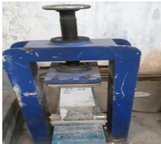
Figure 3 Flexural strength test setup
