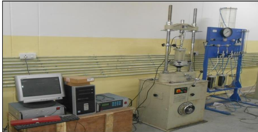
Figure 6 Whole Setup of Triaxial test
