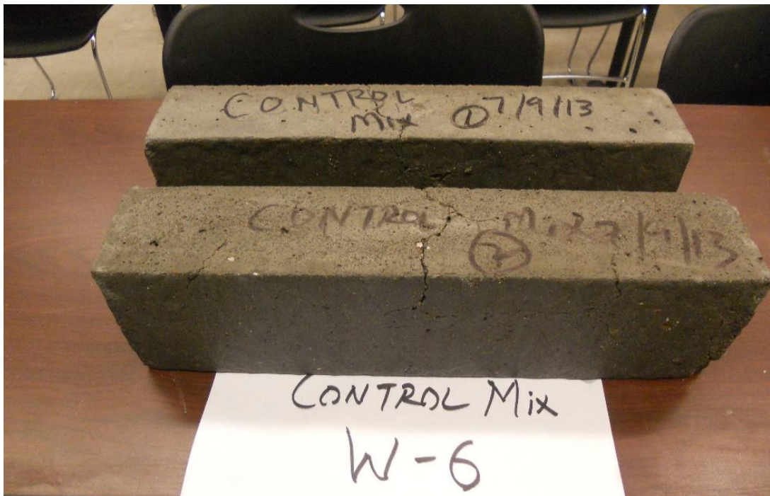
Figure 8 Condition of Control Mix specimen after 6 week (28 day curing)
