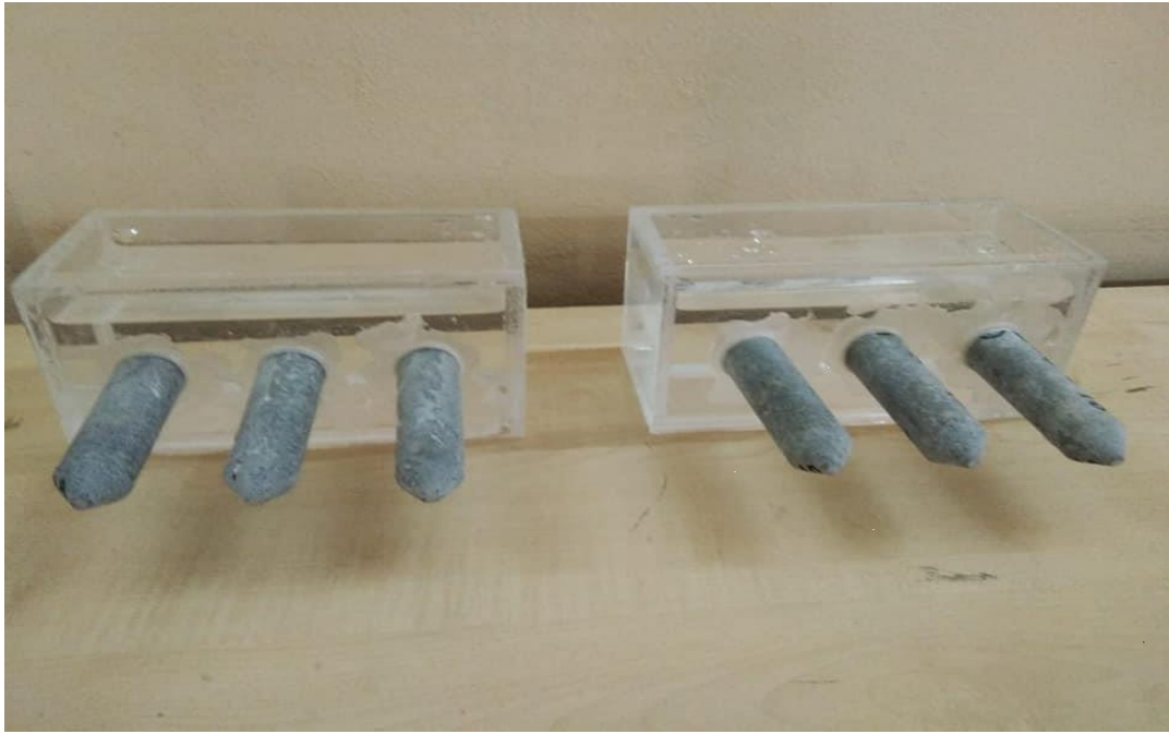
Figure 1 Sample kept in NaCl solution in a box for one dimensional flow
