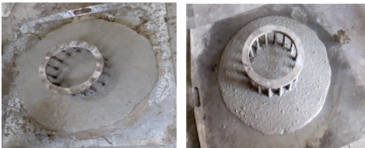
Figure1 (a) J ring for SCC with No fiber content (M0) and (b) J ring for SCC with 1.5 % fiber content (M3)
