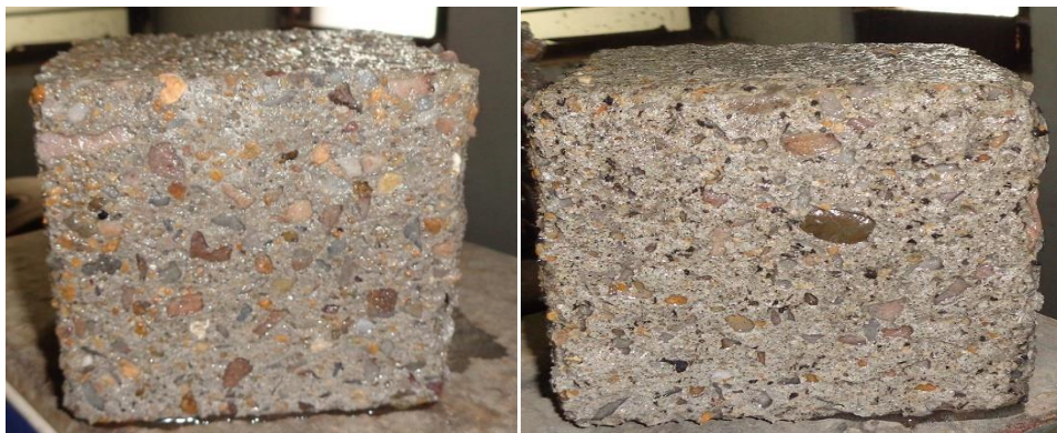
Figure 4: Images of acid attacked specimen at 84 days. The specimen with 0% (left) and 20% (right) crumb rubber
