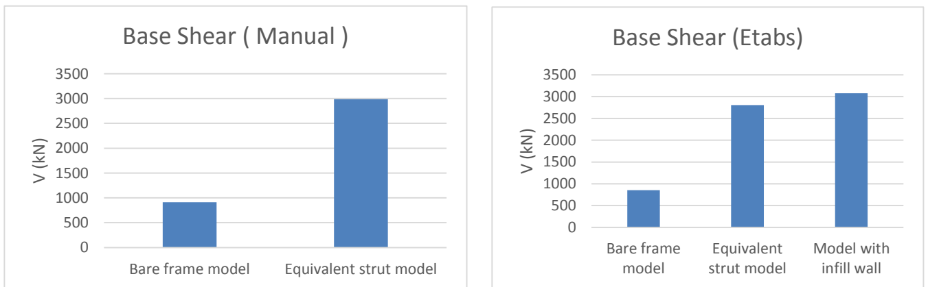
Figure 13 Graph showing comparison of max Base shear values obtained from ETABS and manual calculations
