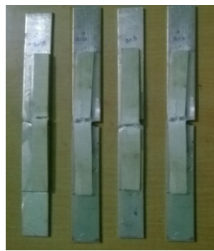
Figure 1 Specimen failure after tensile test
