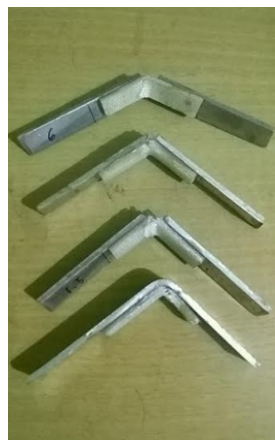
Figure 2 Specimen failure after Flexural Test
