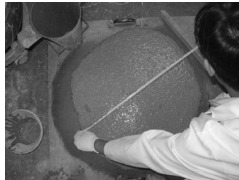
Figure 2 Slump flow for Steel Fiber-Reinforced mix [6]
