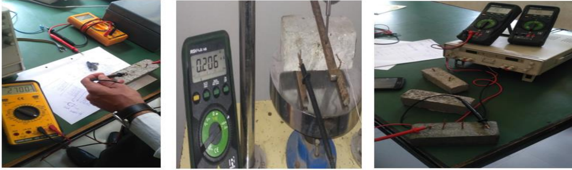
Figure 3 Different cement mortar specimen with different electrical resistivity
