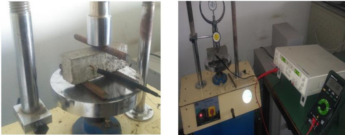
Figure 4 Cement/CNT during three points bending testing with simultaneous electrical resistivity measurement
