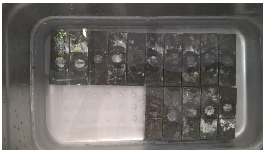
Figure 2: Cracked fibre cement specimens placed in a water bath to heal
