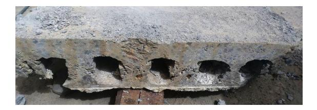
A Lab testing programme on the failed slab (Ref. Appendix A ) revealed that the **concrete quality in SFH 103 was quite variable, with honeycombing & loose, poorly compacted concrete** in some areas, resulting in a poor strand bond. All the 3 strands at one end of the slab were debonded. Both the strands in the slice near midspan had a low bond strength of less than 1 Mpa. Only in the third slice, it took a significant force to push 2 of the 3 strands out of the concrete.
