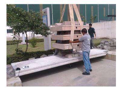
As a result of carrying out this strict selection process on the basis of clearly defined objective criterion, 37 HC slabs were rejected while the rest were cleared for erection. The machine manufacturer's engineers were called in who opened up the whole machinery, corrected the necessary settings to produce further HC slabs whose quality was clearly improved.
