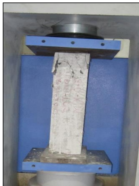
Figure 2 Test set-up of SFRSC Column
