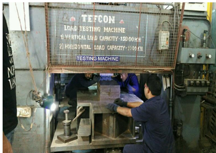
Figure 2 Setup for Axial Compression Test
