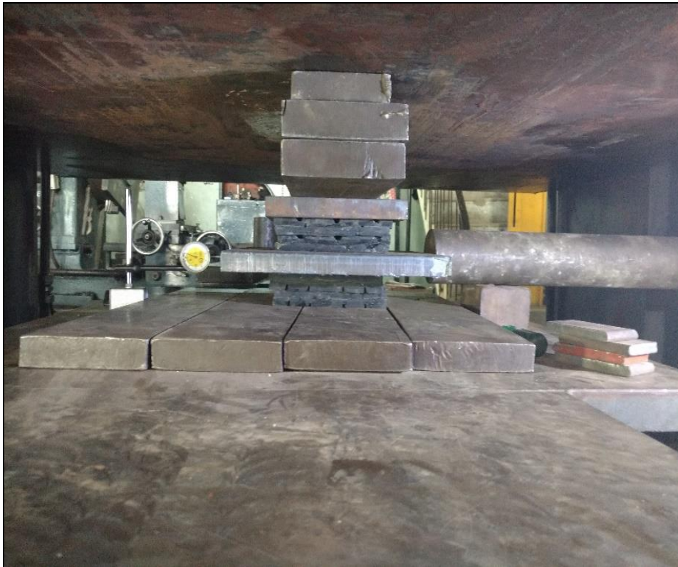
Figure 6 Setup for Horizontal Shear Test on STRP
