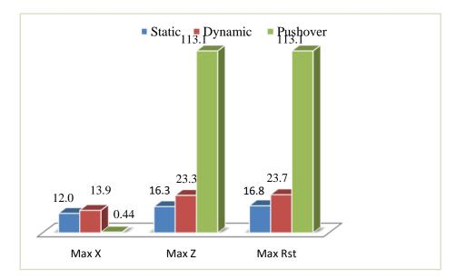
Figure 6 - Comparison of Nodal Displacements, Zone - III
