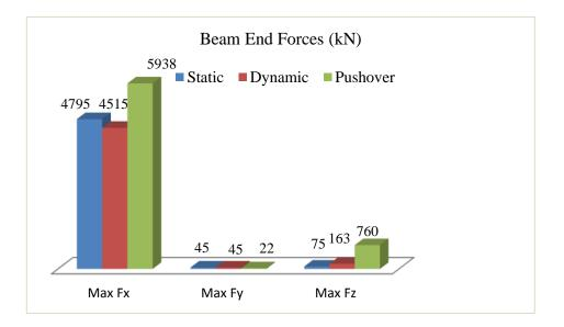
Figure 5 - Comparison of beam end forces, Zone - III
