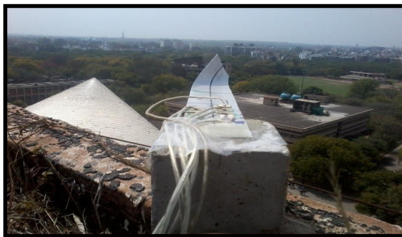
Figure 4 Concept of piezoelectric wind energy harvesting [8].
