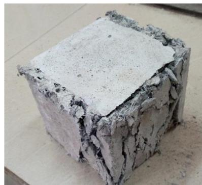
Figure 2 Tested cube at room temperature
