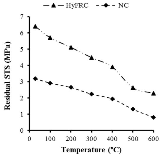
Figure 4 Variation of STS with temperature
