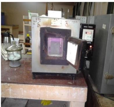
Figure 1 Muffle furnace
