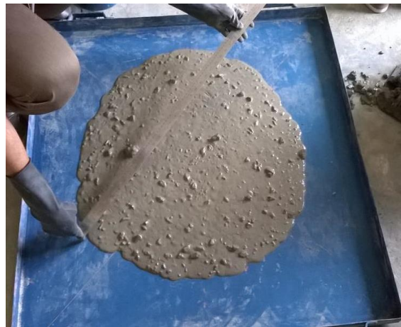
Figure 2 Slump Flow Test for SCC
