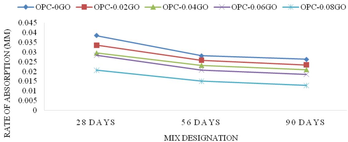
Fig. 6 Initial surface absorption result for all the mixes
