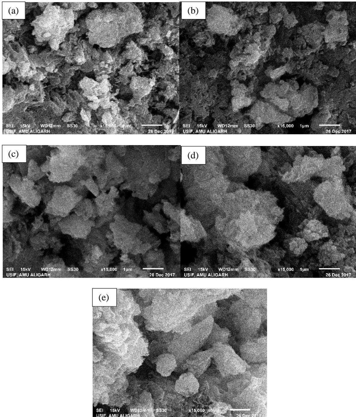
Fig. 8 SEM of mix with (a) GO 0% Control mix, (b) GO 0.02%, (c) GO 0.04%, (d) GO 0.06%, (e) GO 0.08%
