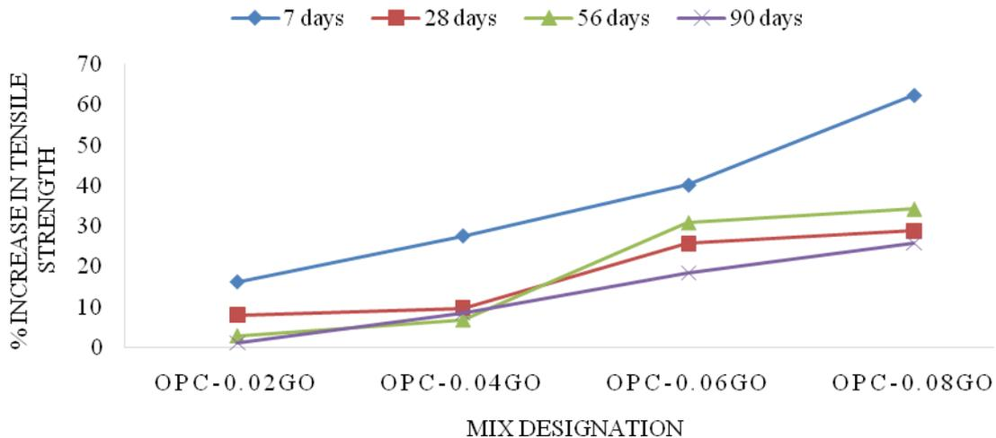
Fig. 4 Percentage increment in tensile strength with respect to control mix
