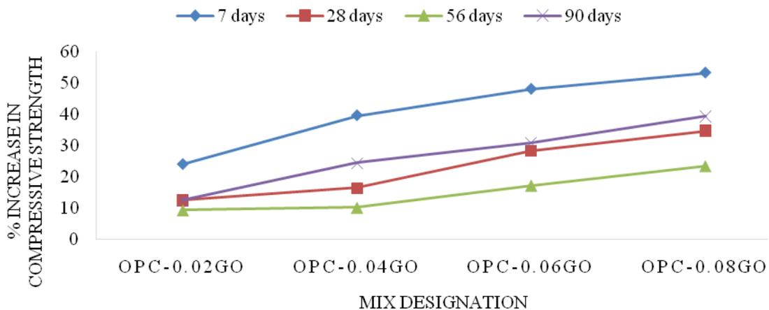
Fig. 3 Percentage increment in compressive strength with respect to control mix
