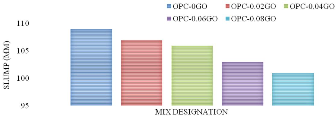
Fig. 2 Slump value of different mixes
