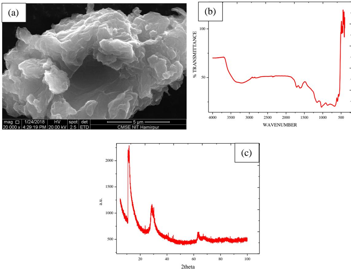
Fig.1 (a) SEM image, (b) FT-IR and (c) XRD of GO
