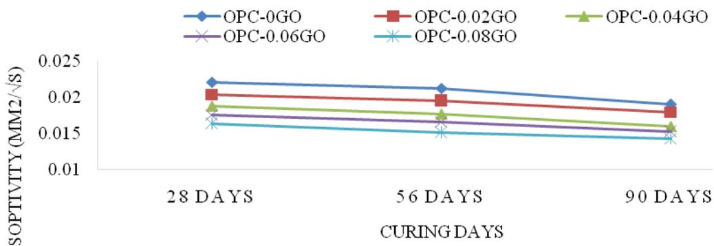
Fig. 7 Initial surface absorption of all the mixes
