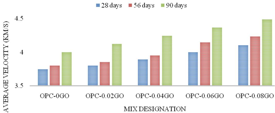
Fig. 5 Ultrasonic pulse velocity of different mixes
