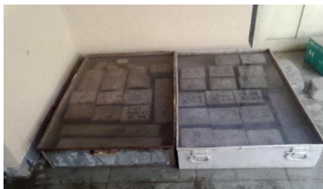
Figure 7 Curing tank with specimen
