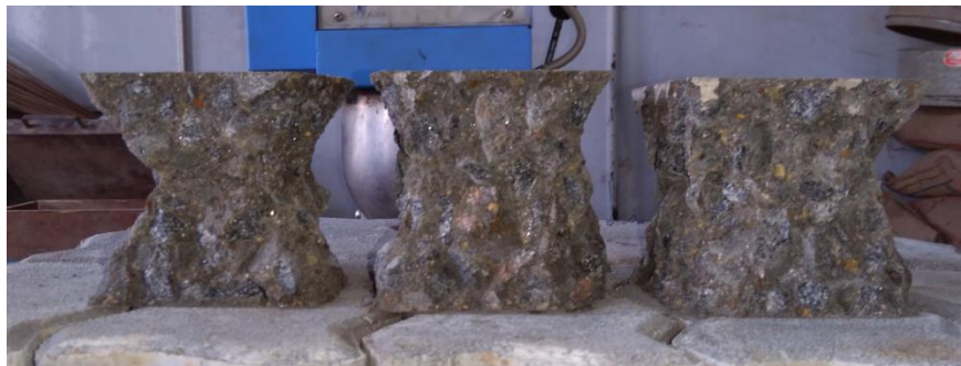
i) concrete with natural aggregates
