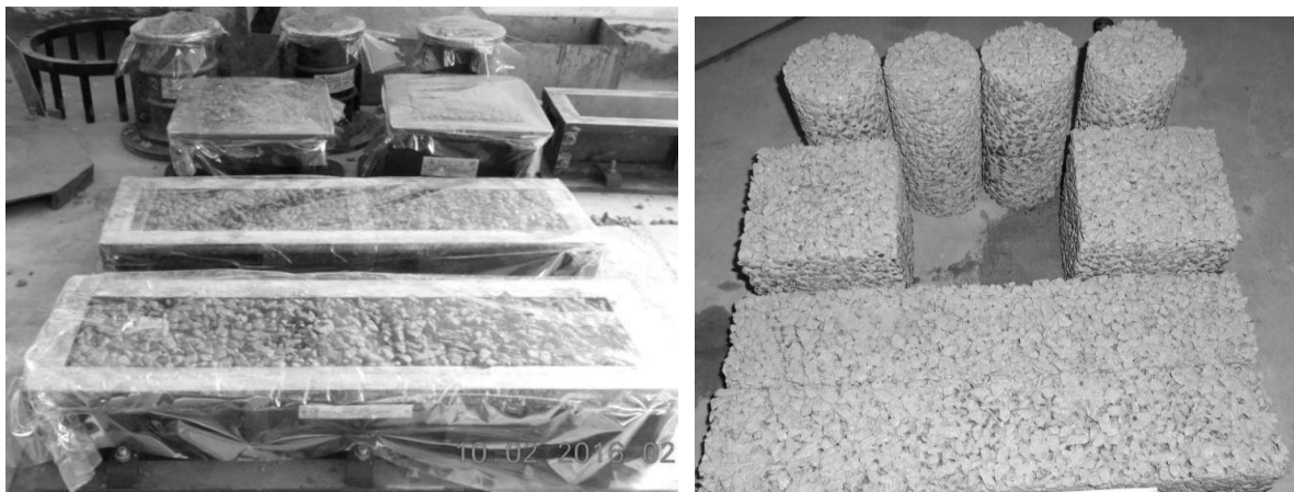
Figure 3 After casting immediately covered the moulds with polythene sheet
