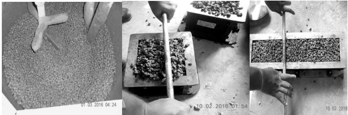
Figure 2 Concrete Mixing & Specimen samples level with steel rod
