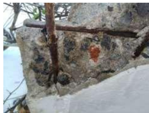
Figure 2 Concrete remains colourless
