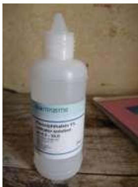
Figure 1 Phenolphthelin liquid used for carbonation test
