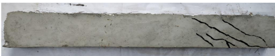
(c) Ferrocement rehabilitated beam (Side view)
