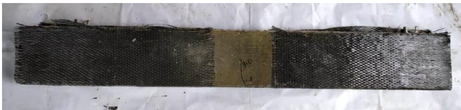
(b) CFRP rehabilitated beam (Side view)
