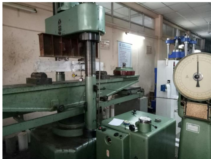
Figure 2 Test setup showing beam specimen with LVDTs and dial gauge
