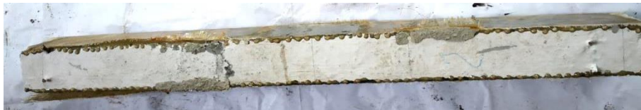
(a) GFRP rehabilitated beam (Top view)
